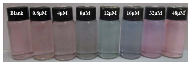
Fig. 3. Color responses when AuNRs react with \text{Cu}^{2+} of various concentrations.
